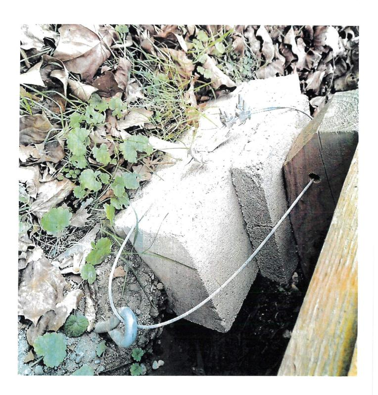
It is important to ensure wire rope clips are installed properly. Incorrect installation can reduce the working load limit by 40%. Below are general guidelines for installing wire rope clips.
