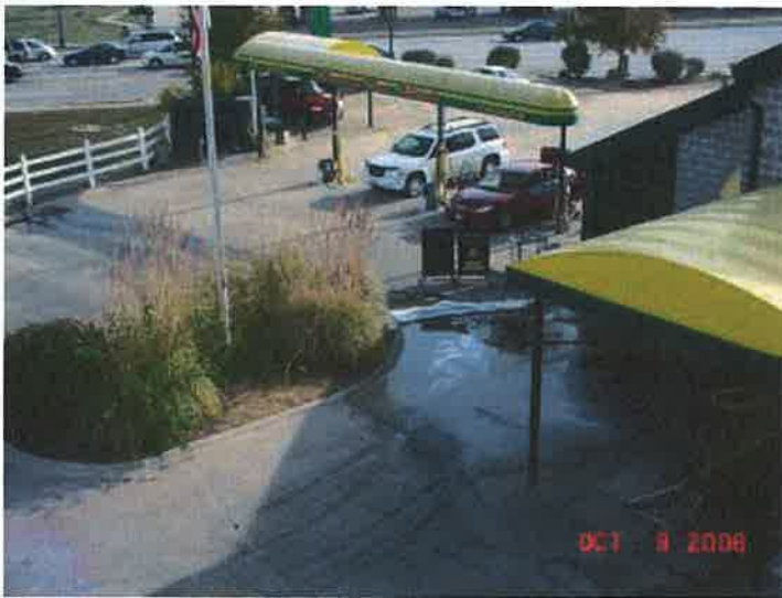
Figure 5: Hot spot Commercial Carwash – overflow directly to storm drain which leads directly to creek
