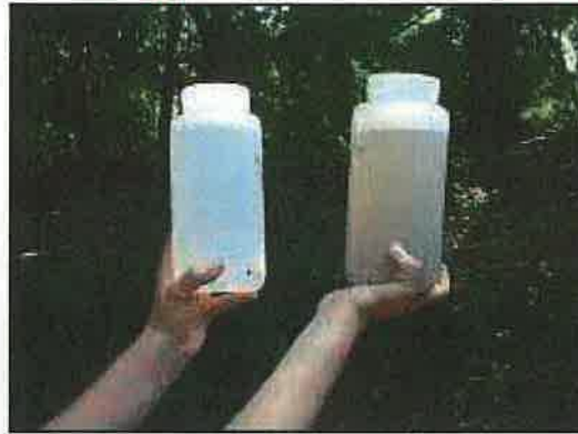
Using a clear sample bottle to estimate color and turbidity
