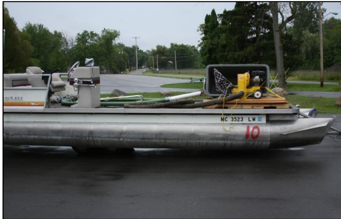
Figure 33. A DASH boat for hand-removal of milfoil or other nuisance vegetation. ©Restorative Lake Sciences
