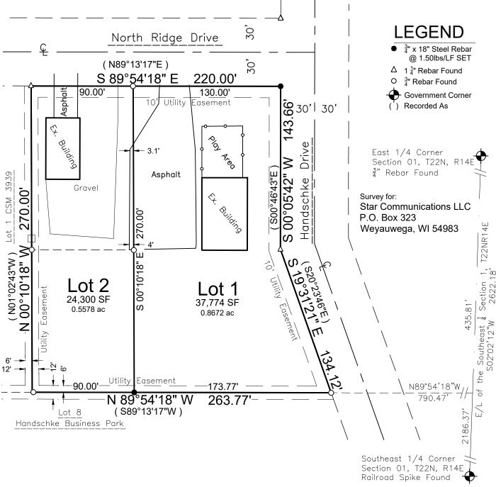
\* There are no pulblished coordinates for Section 01, T22N, R14E, we tied to the South line of Section 36 T23N, R14E, as published, then located the Section Corner monuments shown on this map.
