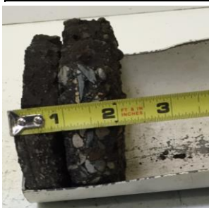
**Core picture shows approximate thickness CORE LOG DCP 1 meter rod (standard).XLS ver. 2/7/14- Clay DCP
