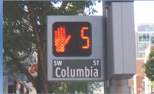
Figure 4.1.4: Pedestrian Countdown Timer (Portland, OR)
