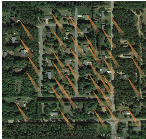
Figure 19. (Right) Picture of subdivision with homes served by private wells and septic system drainfields. Groundwater flow direction is from upper-left to lower-right. Orange shapes illustrate hypothetical plumes paths downgradient of drainfields. Lawn fertilizers in excess of what the lawn is able to use may also represent a source of nitrate to groundwater in these settings.
