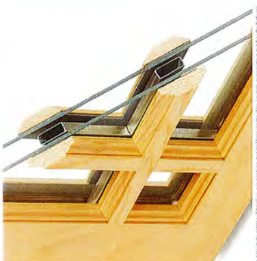
Close-up of a window frame showing the internal structure and glass panes.
