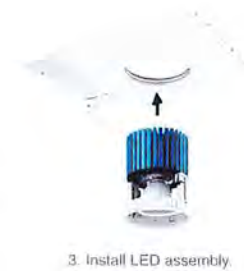
3. Install LED assembly.
