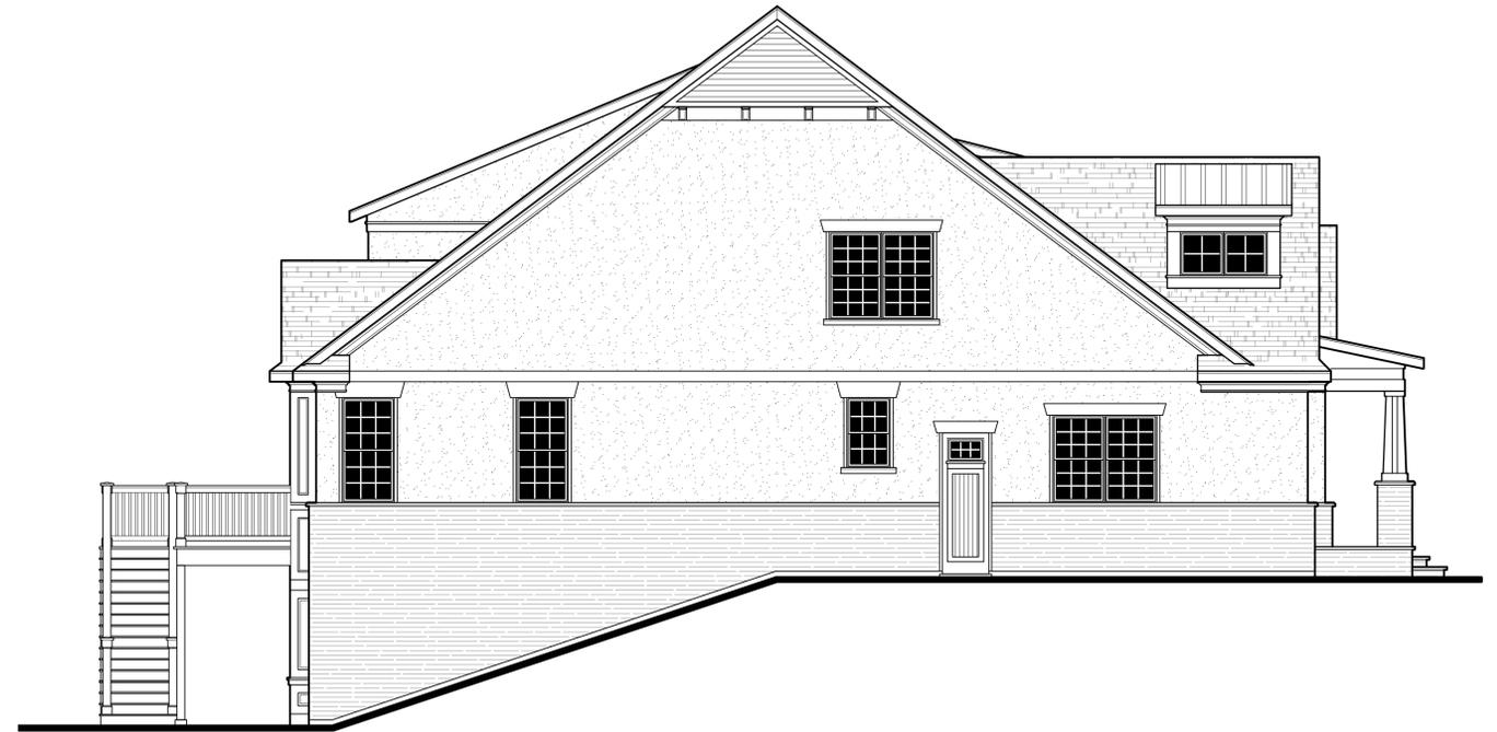
**Side (Left) Elevation - Walkout Condition**
