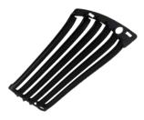
Flush mounted Front Side Shield cuts light off at approximately 1½ times the mounting height in front of the luminaire (street side) and 2¼ times the mounting height laterally.
