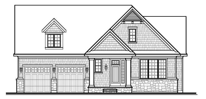
The vertical height of the new plan is approximately 27' 2" from the top of the highest foundation point to the roof ridge, which is slightly higher than the current ranch plan, but of course less than the height maximum of the two story plans of 31 34'.
