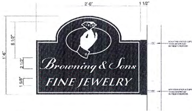
ONE (1) D.F. NON ILLUMINATED BLADE SIGN DISPLAY 1 1/2" = 1'-0" FLAT ALUM. BLADE AND BRACKET PAINTED DURANDIC BRONZE. GRAPHICS TO BE WHITE VINYL.
