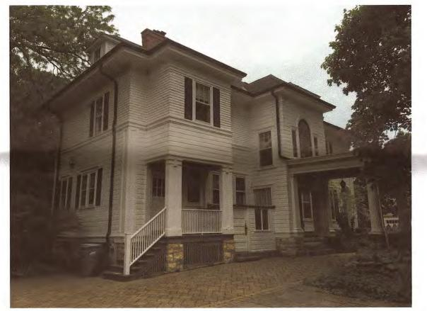
6 - North-west corner showing kitchen entance with double columns covered porch. Narrow double hung windows with louvered shutters. North brick chimney shown.
