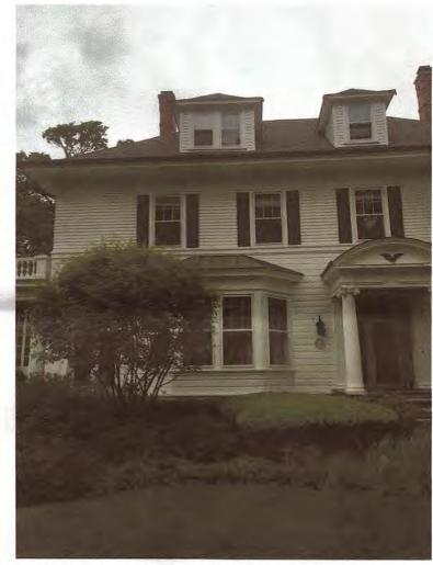
4 - East elevation showing hipped roof with dormers. Bay window at first floor. First floor windows feature 9 panels at upper sash and second floor window s, 6 panels at upper sash.
