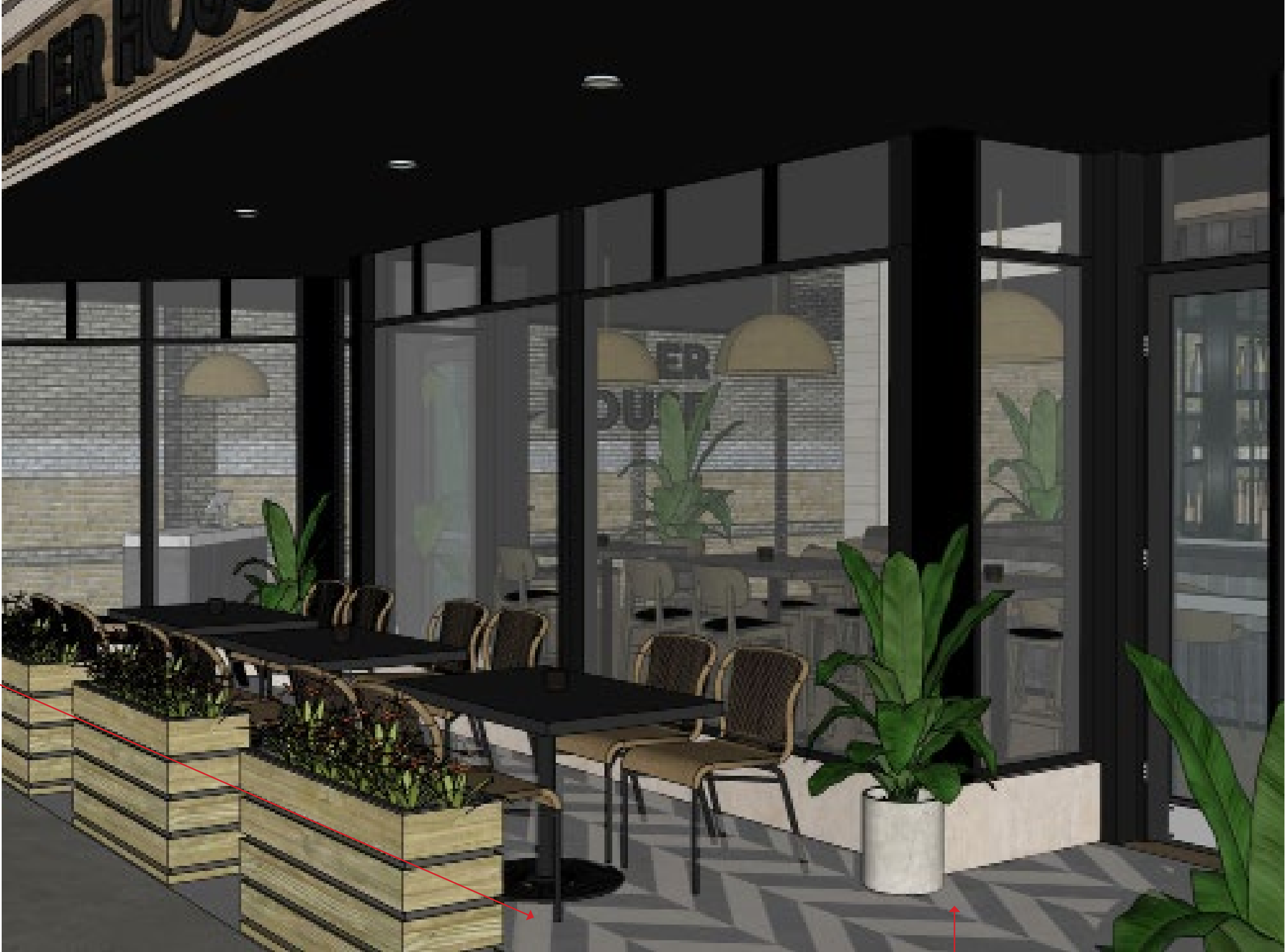
APPLIED PAINTED & SEALED PATTERN STENCIL ONTO EXISTING CONCRETE AT ENTRYWAY TO DISGUISE TRAFFIC WEAR (SEE PROPOSED CONCRETE STENCIL REPEAT PROVIDED)
