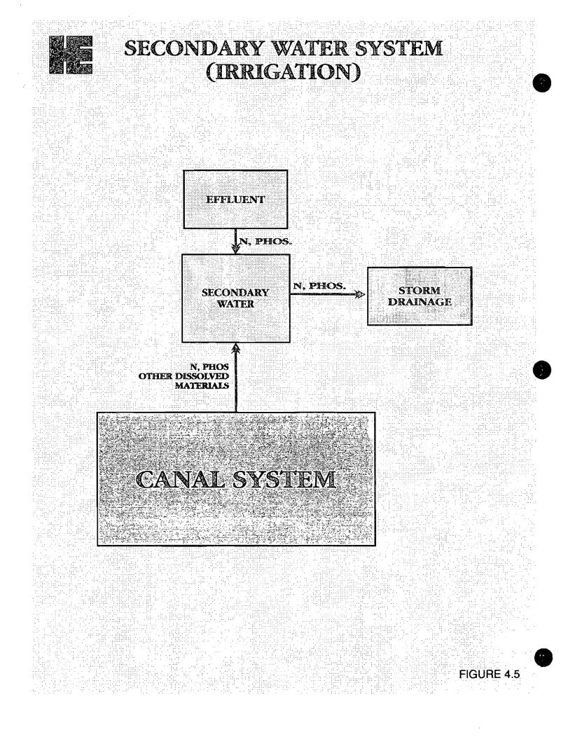
Canal water availability must be reliable for the secondary water system to be effective. The study will analyze the impact of proposed secondary water pumping station locations as well as contingent intakes to assure a high degree of canal water reliability. (See Appendix A.3)
