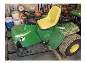
**Description:** Ballfield Machine/Bunker Rake
